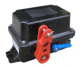
Emergency pull cord switches are used to rapidly turn off conveyor belts or other large machinery and equipment by pulling the line connected to a switch. An emergency pull cord switch serves for personal protection e.g. falling on the conveyor, caught in machinery, pulling a line, etc.
