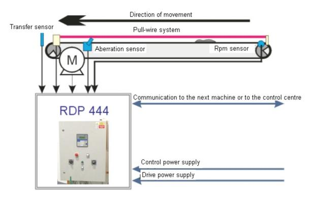
The figure above shows the schematic diagram for an optimum connection of the RDP 444 unit. The most suitable position of the unit is close to the conveyor drive. The position is determined by the cabling for the drive. The sensors are connected according to the diagram; the longest path is that of the rpm sensor which will be installed on the angle pulley. If the drive is on the opposite side of the conveyor than in the diagram, the transfer sensor will represent the same distance.
